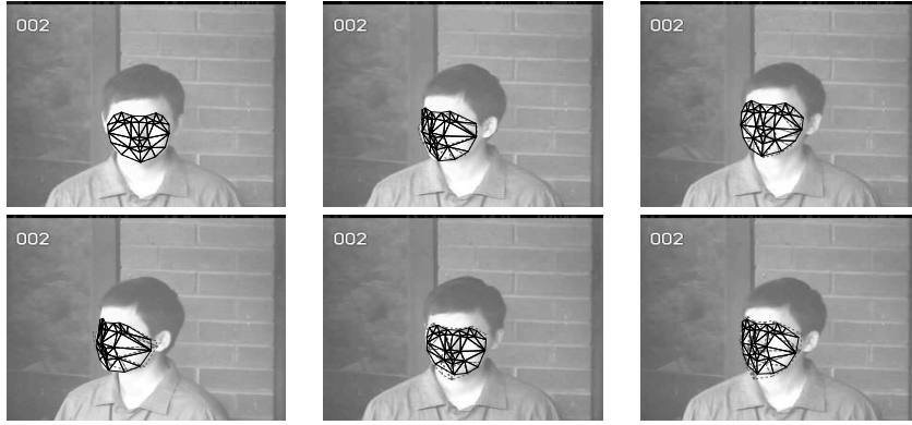
Figure 4: Comparison of the fitted mesh using the SICOV algorithm (dashed line) and the conventional SIC algorithm (solid line) on 6 frames (frame 1, 40, 87, 287, 734 and 767).
