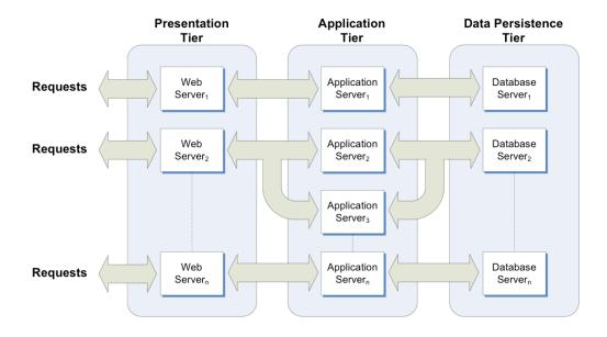
Figure 1: Multiple application architecture.
