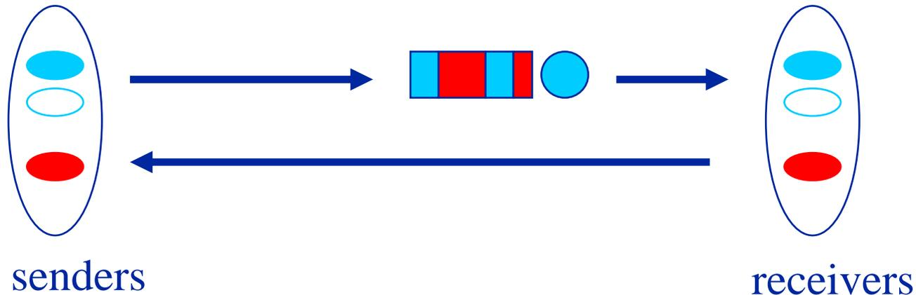
Senders learn (through feedback from receivers) of congestion at queue, and slow down or speed up accordingly. With current TCP, throughput of a flow is proportional to
