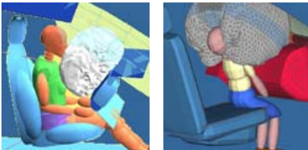
Figures 5 and 6. Impact and airbag delivery for a belted female adult and an unbelted child.
