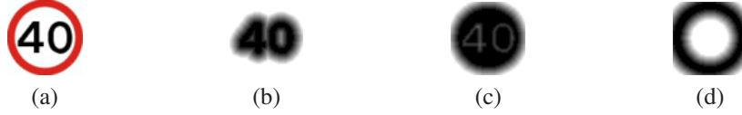
Figure 3: Colour Distance Transform images: original discrete colour image (a), black CDT (b), white CDT (c), red CDT (d); darker regions denote shorter distance.
