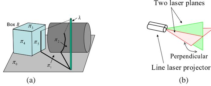
Figure 2: Metric constraints of coplanarities in a scene:(a) Rectangular box with shadow of straight bar.  $\pi_0 \perp \pi_1$  and  $\pi_0 \perp \pi_2$  if  $\lambda \perp \pi_0$ .  $\pi_3 \perp \pi_4$ ,  $\pi_4 \perp \pi_5$ ,  $\pi_3 \perp \pi_5$ , and  $\pi_3 \parallel \pi_0$  if box  $B$  is rectangular and on  $\pi_0$ . (b) A laser projector with two line lasers.
