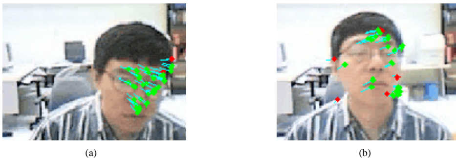
Figure 3: Two examples of outliers among the feature points. The cyan lines indicate the features' positions in the previous frame. The red dots are outliers and the green dots inliers w.r.t. the computed fundamental matrix. The outliers will be removed from the point set.
