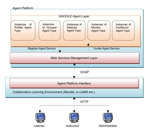
**Figure 6**: Architecture of integrating GAOOLE agents in a CLE
