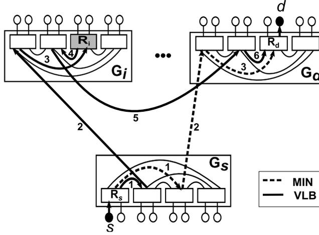
Fig. 3. MIN and VLB routing on Dragonfly
