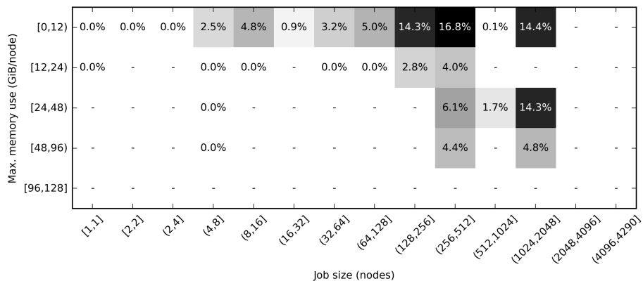
Fig. 5. Usage heatmap of maximum memory versus job size for SBLI jobs in the period.
