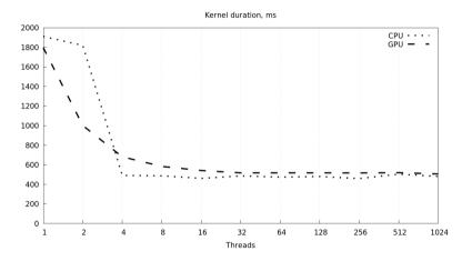
NVIDIA Tesla K20c GPU vs. Intel Xeon E5-1620v2 CPU (4 cores).
