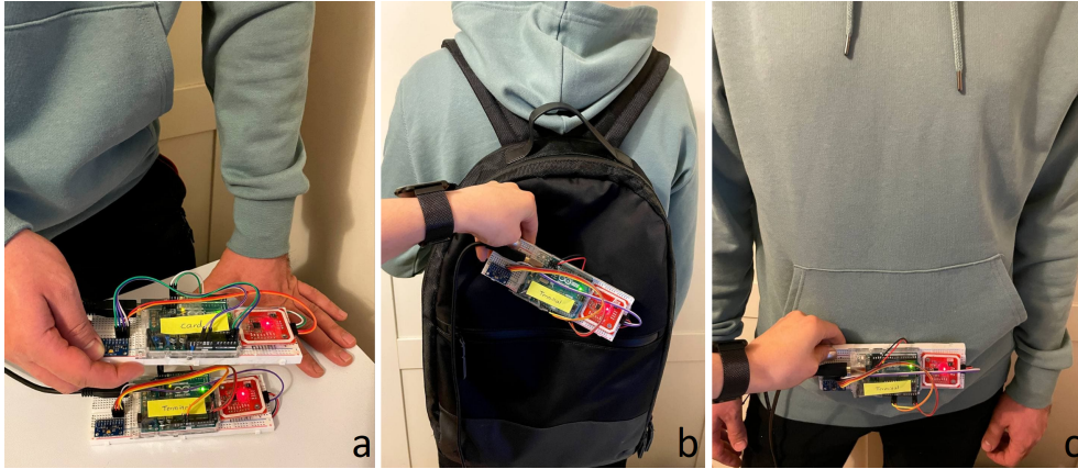
Figure 5.5: User Study Setup: a) OPay Payment Setup; b) Random Guessing Attack; c) Targeted Guessing Attack
