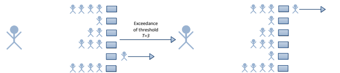
Fig. 4. Departure redirection for the lower bound model; SQ(2), N = 6 servers, and threshold T = 3
