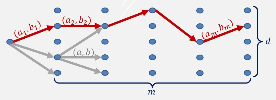
The samples  $(a_1, b_1), \ldots, (a_m, b_m)$  define a computation-path. Each vertex v in the last layer is labeled by  $\hat{x}_v \in \{0,1\}^n$ . The output is the label  $\hat{x}_v$  of the vertex reached by the path
